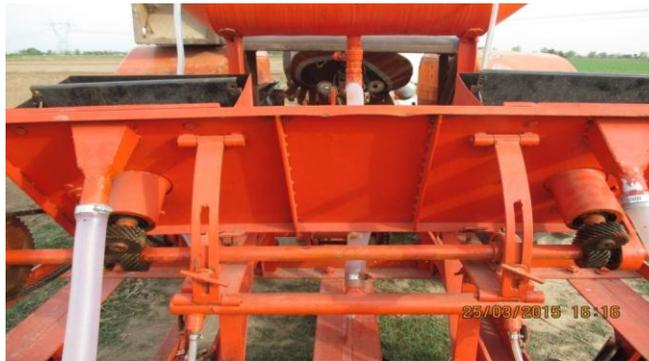
Fig. 6. Central pivot system with seed plate drive mechanism
