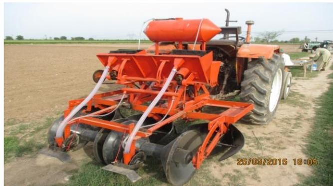
**Fig. 8. Liquid fertilizer application system with double reservoir**
