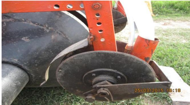
Fig. 7. Furrow opener with seed drop chute
