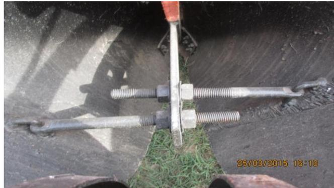
Fig. 3. Ridger wings with hinges and struts
