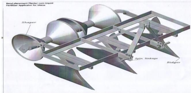
**Fig. 8. Ridge shaper with ridgers and main frame**
